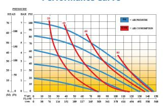
AIR PRESSURE: Tested at 100 psi / 690 kPa (not to exceed 125 psi / 861 kPa) FLOW RATE: 0-146 gpm / 553 Lpm FLUID CONNECTION: 2"/50mm (Internal Thread) AIR INLET PORT: 1/2" / 15mm (Internal Thread) **EXHAUST PORT:** 3/4" / 19mm (Internal Thread) **DELIVERY PRESSURE:** Tested to 87 psi / 60 kPa SUCTION LIFT: Tested to 24' / 7m dry and 30.5' / 9m wet **SOLIDS HANDLING:** 1.8"/46mm PUMP WEIGHT: Yellow Series - 51lbs / 23.1kg Red (FRAS) Series - 60lbs / 27.2kg Blue Series - 42lbs / 19kg
