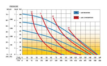
AIR PRESSURE: Tested at 100 psi / 690 kPa (not to exceed 125 psi / 861 kPa)
