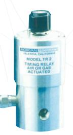
The Morgan TR2 Pneumatic Timing Relay supplies an air/gas pulse that allows a pneumatic SiA or Morgan chemical injection pump to cycle once. By adjusting the time delay between each pulse the TR2 is capable of adjusting the cycle rate of the CIP between 5 and 50 cpm thus varying the flow rate.
