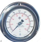
Every gauge is designed to withstand 300% full scale pressure without rupture of the bourdon tube and 130% of full scale pressure without loss of accuracy.
