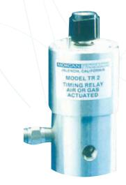
The Morgan TR2 Pneumatic Timing Relay supplies an air/gas pulse that allows a pneumatic SiA or Morgan chemical injection pump to cycle once. By adjusting the time delay between each pulse the TR2 is capable of adjusting the cycle rate of the CIP between 5 and 50 cpm thus varying the flow rate.
