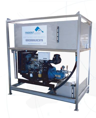
Trident Australia diesel driven Hydro Pressure Unit. Perkins diesel motor coupled to Hughes pump can be used for a variety of applications including pressure testing, pressure cleaning and general hydrostatic work. Manually adjusted pressure control valve allows output pressure to be controlled and set quickly for each application.
