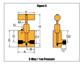
G - Packing gland mounting hole drill size
