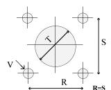
1/4" - 1/2" VALVES ARE M4 x 6 mm DEEP 3/4" VALVES ARE M5 x 6 mm DEEP 1" - 1.1/4" VALVES ARE M6 x 8 mm DEEP 1.1/2" - 2" VALVES ARE M8 x 8 mm DEEP
