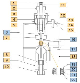
150V Shutoff torque = 32 ft-lbf (Force in excess could damage stem)
