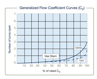
100VM and 150V Series Flow Curve for Vee Stem Valves
