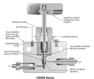
Note: 100VM9 Series comes with a T-Handle. To ensure proper fit use Parker Autoclave tubing
