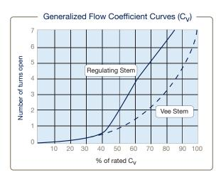
30SC and 43SC Series Flow Curve for Vee and Regulating Stem Valves
