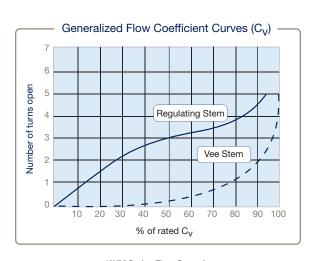
40VM Series Flow Curve for Vee and Regulating Stem Valves
