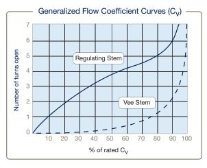
30VM Series Flow Curve for Vee and Regulating Stem Valves
